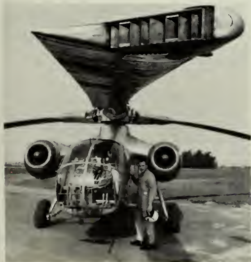
HOT CYCLE research helicopter now under development gets power from hot gases jetted through tips of rotor blades.
